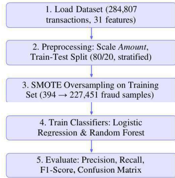
Fig. 2. Proposed fraud detection pipeline from raw data to model evaluation.
